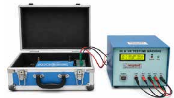
IR & VR Testing Machine
